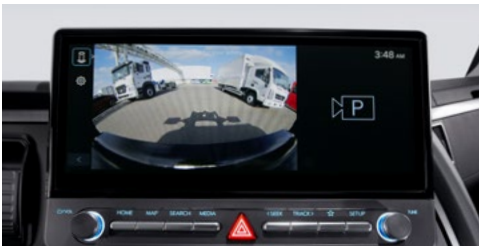
Rear View Monitor Equipped with an extra-wide-angle lens, the screen provides a real-time rear view video feed.
