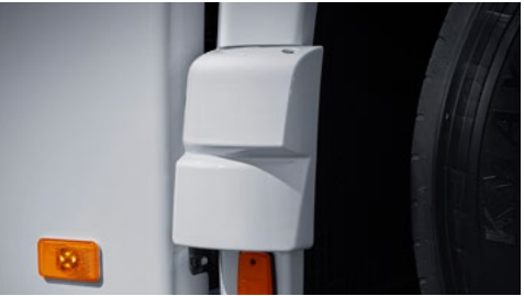
Side-Front Sensor and Side-Rear Sensor Side-front and side-rear sensors enhance safety by detecting blind spots and preventing accidents during reversing and lane changes.
