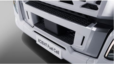
Elongated Bumper Rounded corners and an elongated bumper reduce air resistance, enhancing aerodynamic performance by 2.8% and fuel efficiency by 1.2%.
