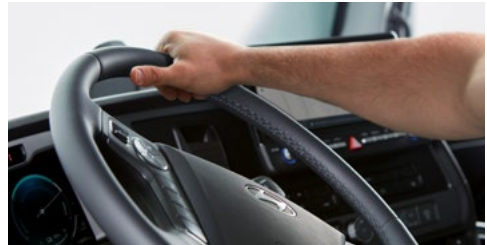
Motor Assist Hydraulic Steering (MAHS) At a higher speed, MAHS provides a heavier steering feel for improved stability, while at a lower speed, the wheel feels lighter for easier turning and parking. (optional)
