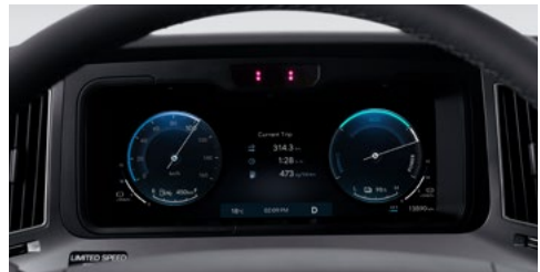
12.3-inch Digital Cluster Providing all the essential information with minimal distraction, the 12.3-inch cluster features sharp, easy-to-read graphics.
